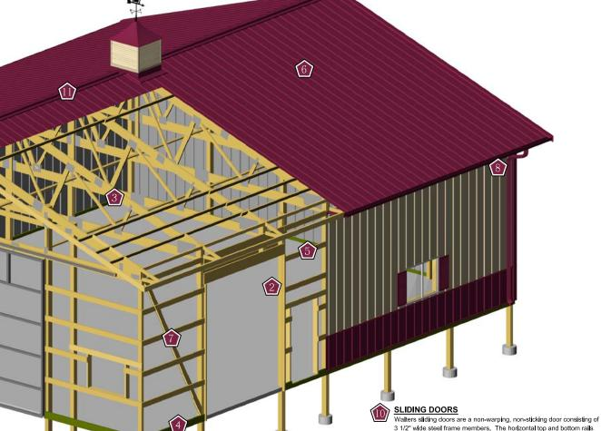
3 1/2" wide steel frame members. The horizontal top and bottom rails and the vertical rails are made of 16ga G-90 Galvanized steel. The intermediate horizontal rails are made of 20ga G-90 Galvanized steel. Door latches are located at the center on a double door and at the iambs on all doors. These latches are designed to be latched in either the open or closed postition. Latching the door in the open position prevents wind blowing door to a half open position, causing damage.
